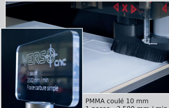
PMMA coulé 10 mm
